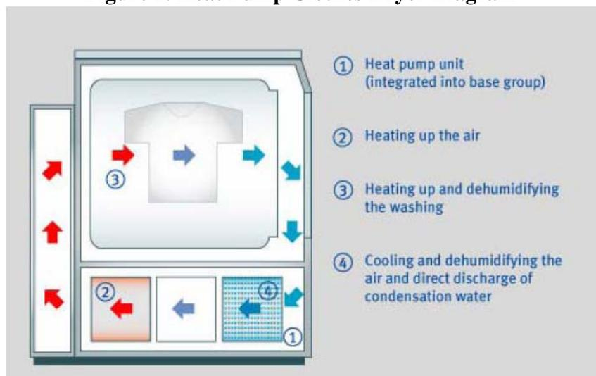
A heat pump delivers heat by extracting energy from the ambient air. The hot dry processed air enters the rear of the drum and interacts with the laundry. Warm moist air exits the drum and proceeds through the lint screen and through the evaporator where a significant portion of the moisture is removed before flowing through the condenser and back into the drum.
