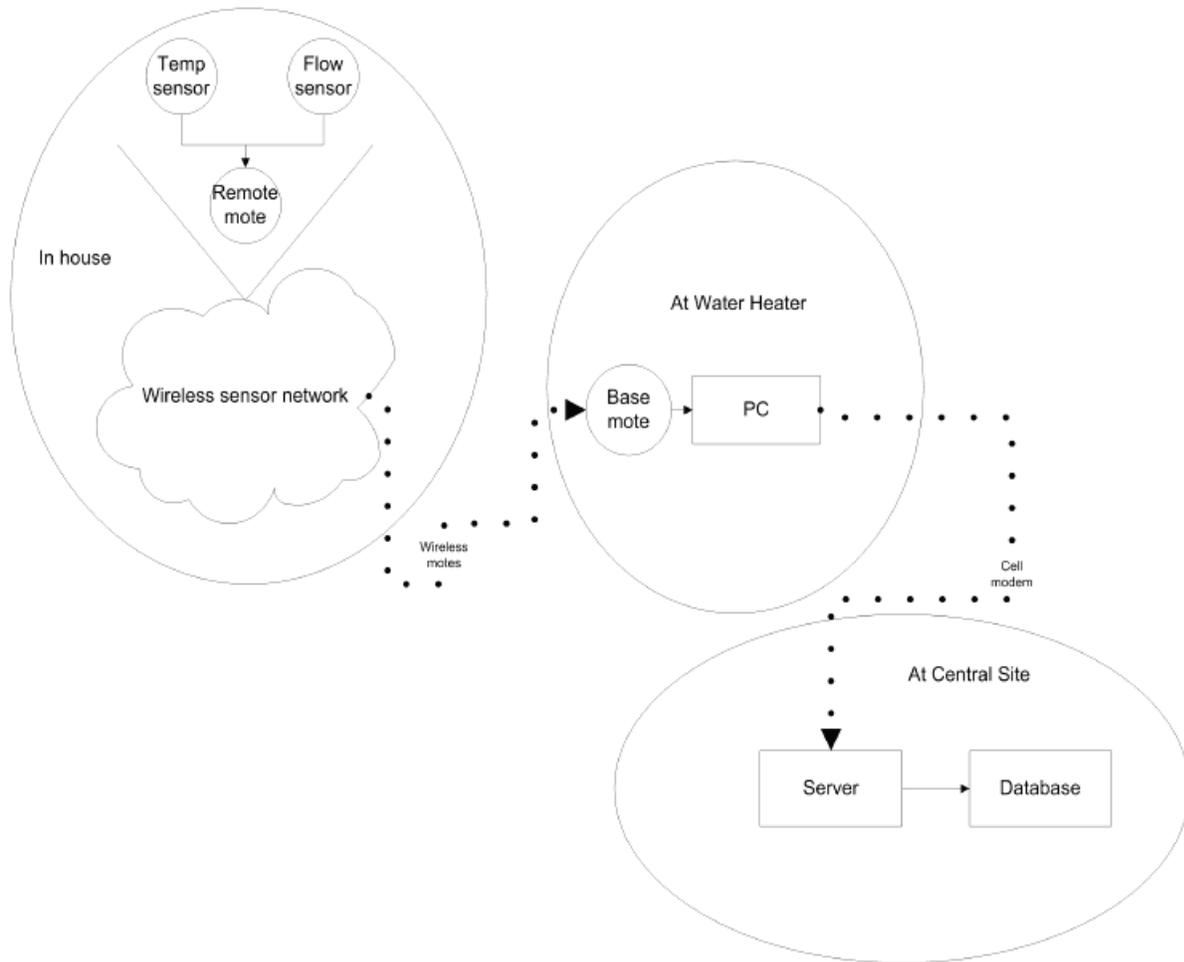
**Figure 3. Wireless data acquisition system.**
