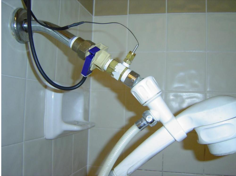
*Figure 5. Flow and temperature sensors installed at showerhead.*
