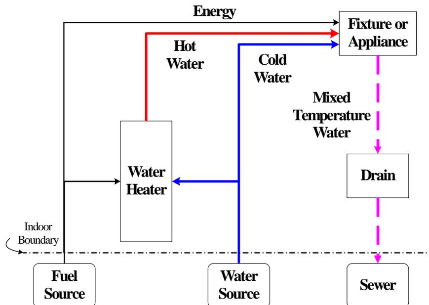
Figure 1. Typical residential hot water distribution system.
