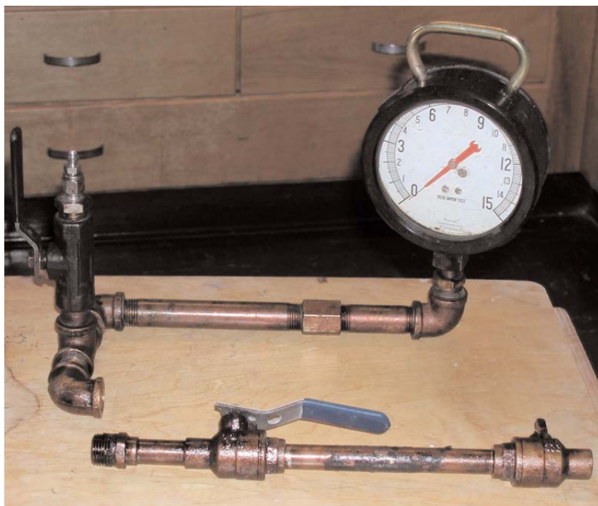
Figure. Oil-sampling device developed for heavy oil tank emissions test.
