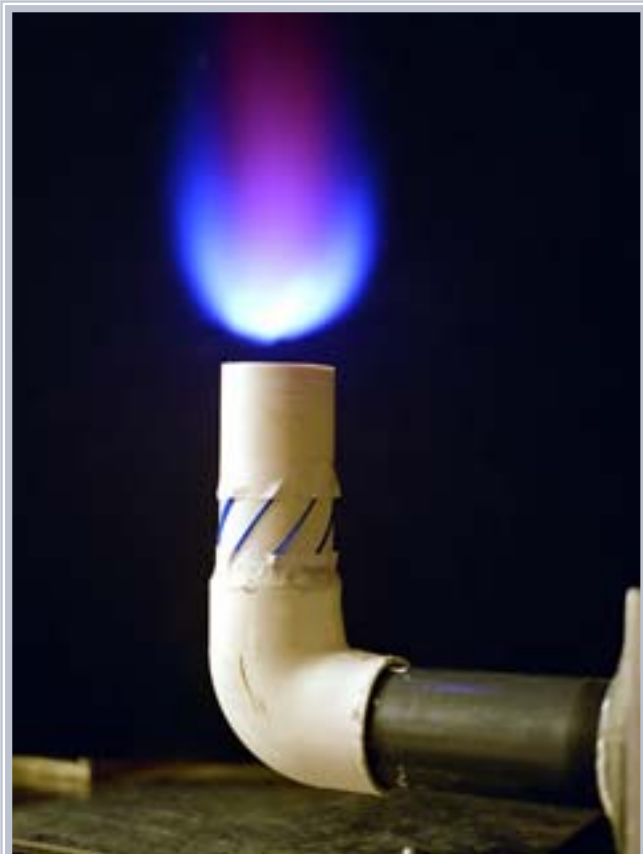
Burner made of PVC to showcase the uniqueness of the LSC concept
